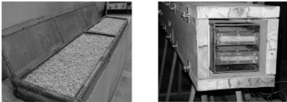
Fig. 2. Gauze holders with poured rice grain and their arrangement in the channel of the large laboratory setup.
